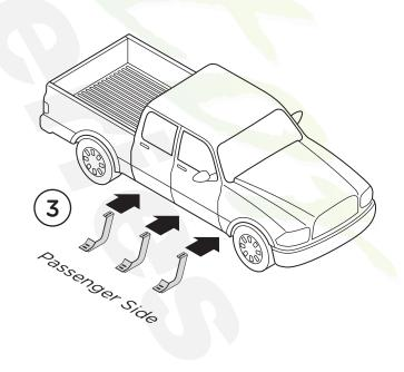
**4.** All passenger side Brackets are identical with the bracket cradle facing toward the rear of the vehicle. Install the first passenger side Bracket closest to the front wheel. Align with existing factory holes in the rocker panel as shown (4a), Secure the first Bracket using one (1) M8 x 30mm Hex Bolt, one (1) M8 Lock Washer and one (1) M8 Flat Washer (4b).
