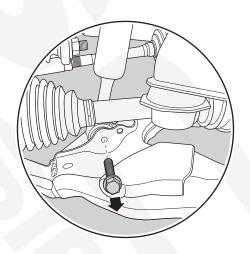
7. Once unbolted slowly lower the factory coilover through the upper control arm, you might have to raise the upper control arm and gently push down on the lower control arm to give enough room for the factory coilover to be removed.
