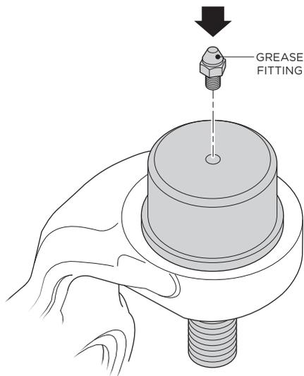
**19.** Install grease fitting into new lower ball joints.
