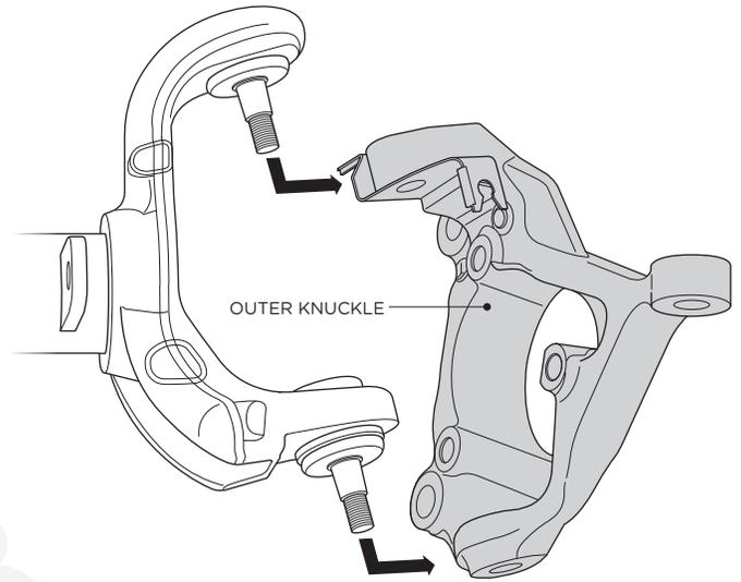
**14.** Remove the upper ball joints and then the lower ball joints by using a ball joint press.
