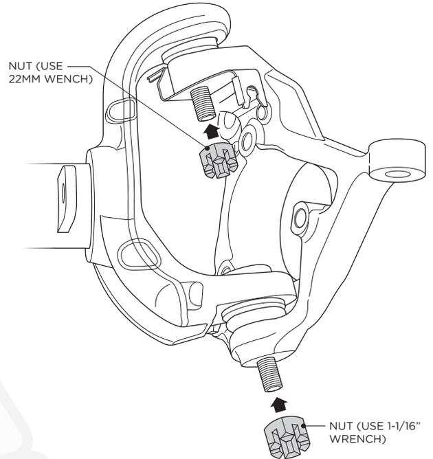
22. Install the cotter pins. Complete the assembly of the ball joint install by reversing steps 1-11.
