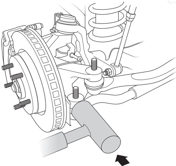
3. Next, remove the rod ends from the knuckle.
