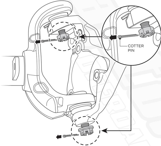
**13.** Use your preferred method when removing the outer knuckle. (Large hammer, pickle fork, etc.)
