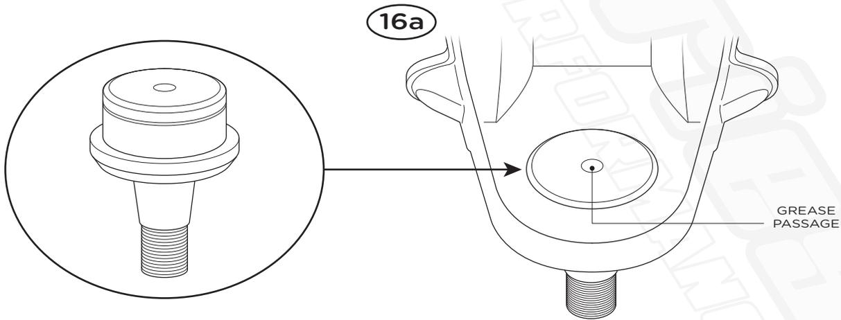
**17.** The orientation of the lower ball joint on the passenger side must be to installed the same as the driver side. Firmly press the lower ball joint into the inner C. Secure lower ball joint using a ball joint press.
