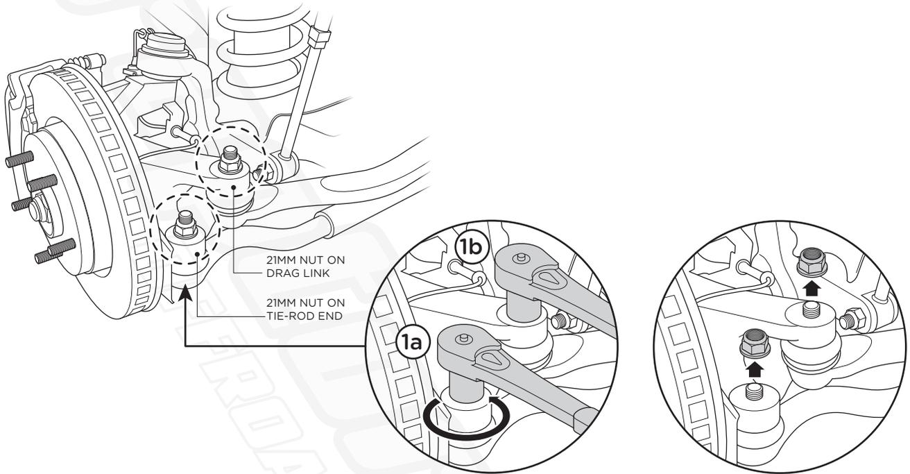
2. Using a hammer, dislodge the tie-rod and drag link ends.
