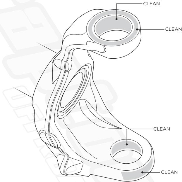
**16.** It is critical to orient lower ball joint correctly.
