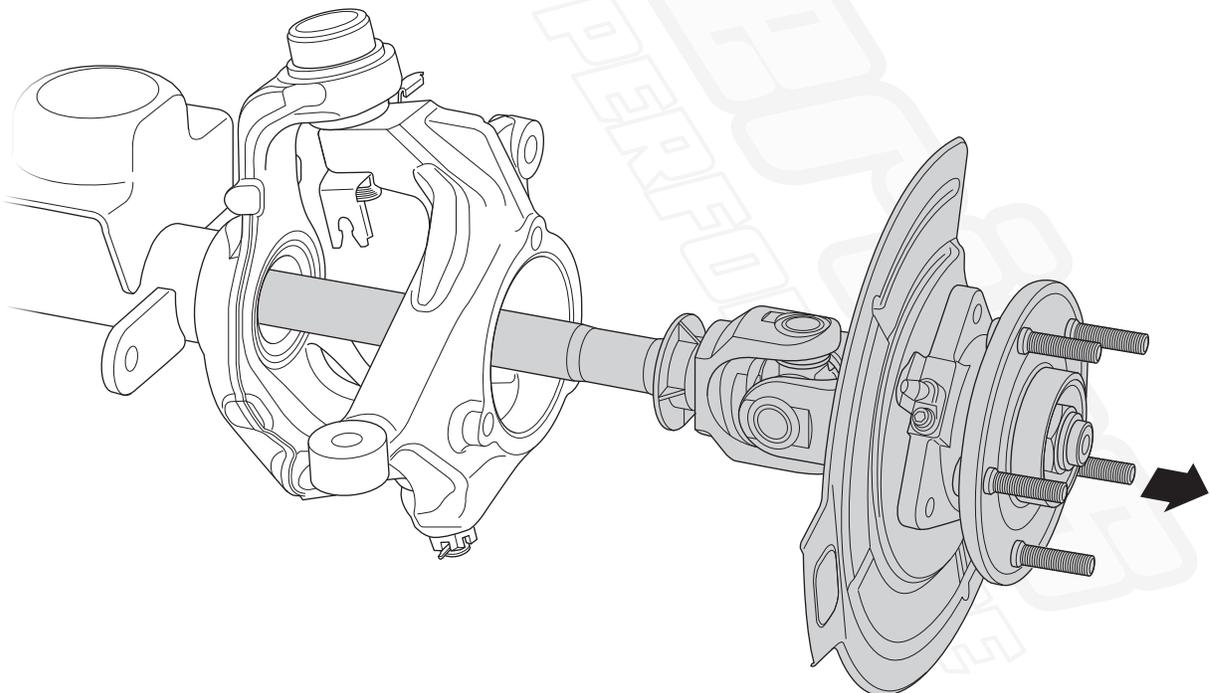
**12.** Remove the cotter pins enabling you to loosen the upper and lower ball joint nuts. Do not completely remove the nuts. This will prevent the knuckle from falling off when it breaks loose from the ball joints.
