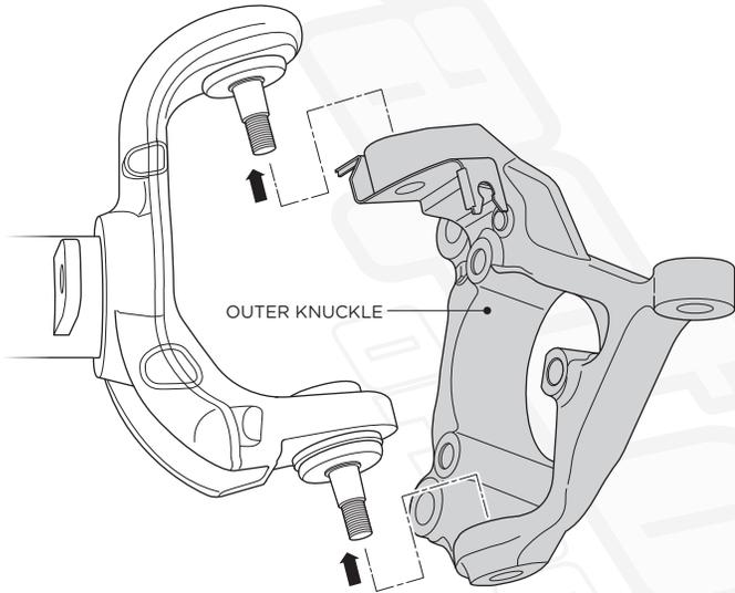
21. Secure the knuckle using the supplied nuts. Tighten the upper ball joint nut using a 22mm wrench and tighten the lower ball joint using a 1 1/16" wrench.
