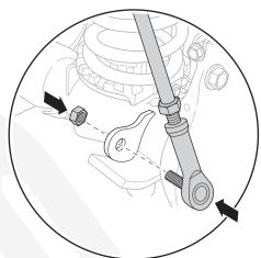
2. Once the sway bar end links are connected, adjust accordingly to reach the ideal sway bar angle shown on page 1. Vehicle must be a normal ride height and located on level ground to accomplish this. Once your sway bar and end links are adjusted correctly, use a 19mm open end wrench on the jam nuts and a 17mm open end wrench on the rod ends to securely tighten the nuts.
