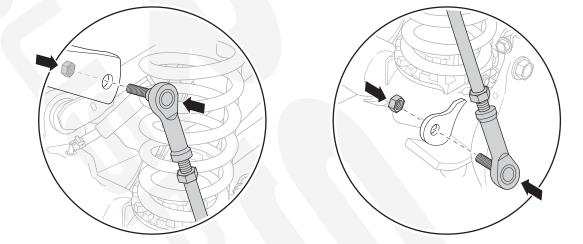
**2.** Once the sway bar end links are connected, adjust accordingly to reach the ideal sway bar angle shown on page 1. Vehicle must be a normal ride height and located on level ground to accomplish this. Once your sway bar and end links are adjusted correctly, use a 19mm open end wrench on the jam nuts and a 17mm open end wrench on the rod ends to securely tighten the nuts.
