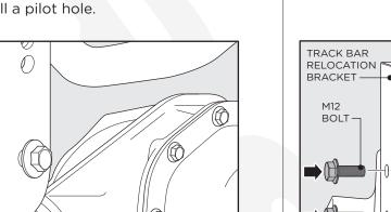
**4.** Install track bar bracket with the provided M12 bolt and M12 nut into the holes just drilled. Do not tighten bolts.
