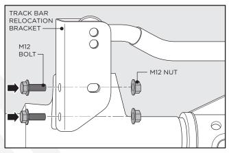
**5.** Install provided M14 bolt, spacer, and M14 nut into track bar relocation bracket and mount. Torque provided M12 bolts to 95 ft-lbs. Torque provided M14 bolt to 150 ft-lbs.
