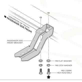
**3.** Fasten the top portion of the Passenger Side Center Bracket by using (2) M8 x 30MM Hex Head Bolts, (2) M8 Flat Washers and (2) M8 Lock Washers.
