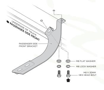
**3.** Fasten the top portion of the Passenger Side Center Bracket by using (2) M8 x 30MM Hex Head Bolts, (2) M8 Flat Washers and (2) M8 Lock Washers.
