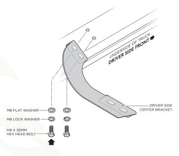
**4.** Fasten the top portion of the Driver Side Rear Bracket by using (2) M8 x 30MM Hex Head Bolts, (2) M8 Flat Washers and (2) M8 Lock Washers.
