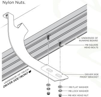
**6.** Fasten the Running Board to the Driver Side Center Bracket cradle by using (2) M8 Flat Washers, (2) M8 Lock Washers and (2) M8 Nylon Nuts.
