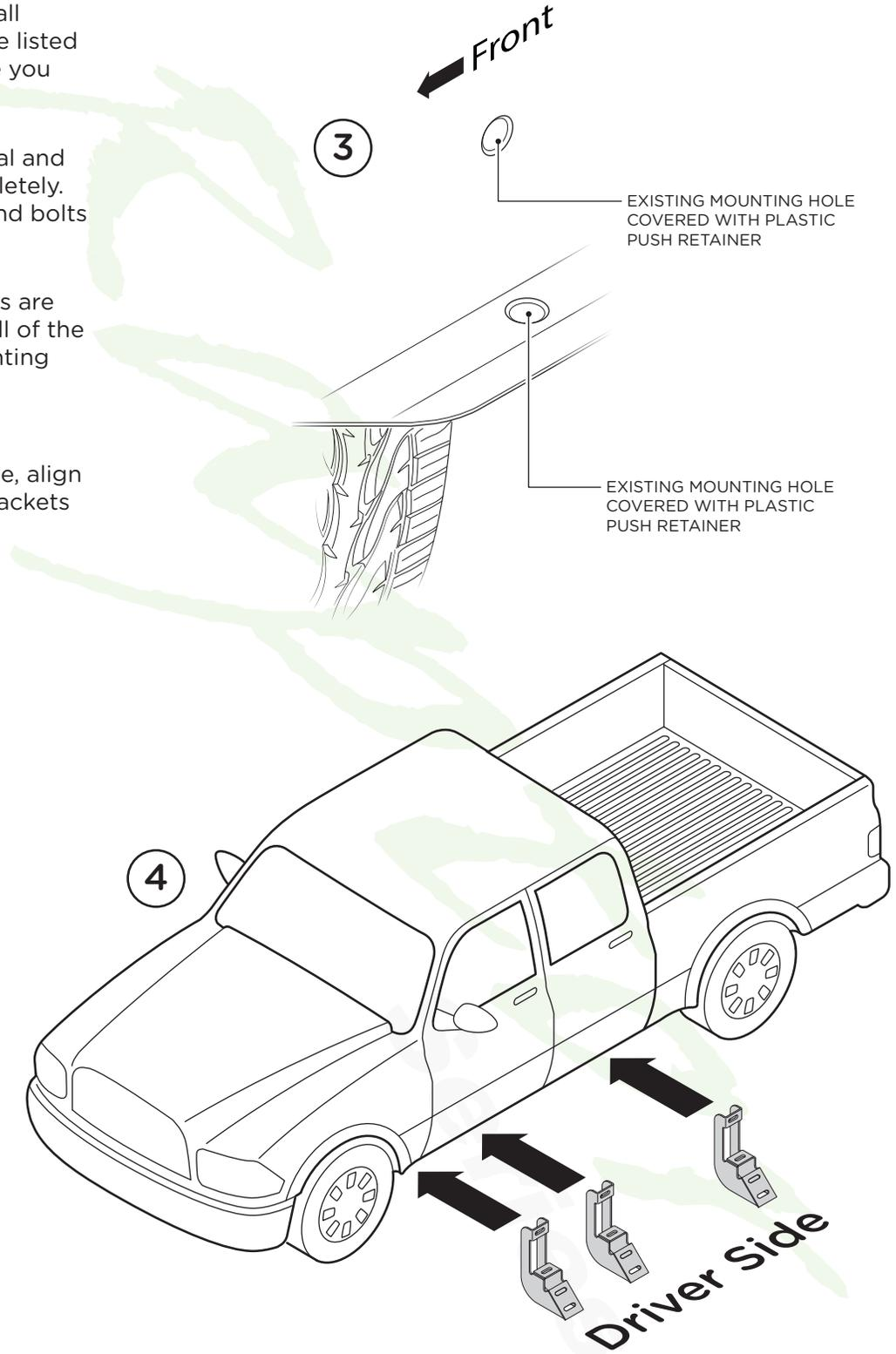
**5.** Starting from the front of the cab, locate the first, third and fifth set of plastic push retainers on the rocker panel. Remove the retainers using a Retainer Removal Tool. This will expose threaded inserts on the rocker panel used for mounting the brackets to the vehicle.
